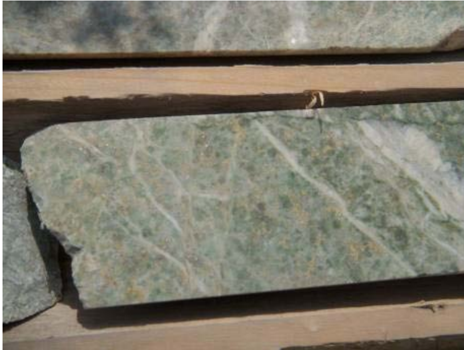
Figure 5: Angel Hill core sample showing gold mineralization.
